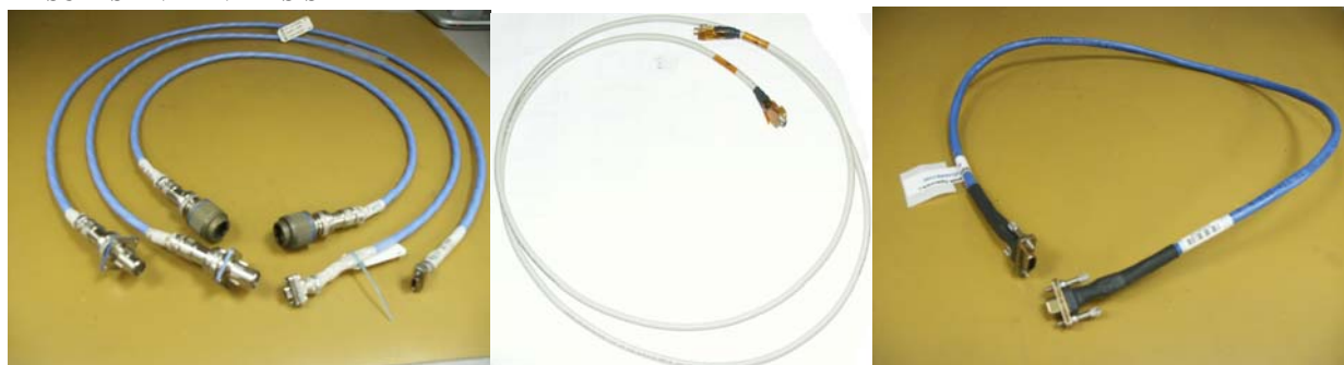
Figure 2: Picture showing the flight (left, in unmounted configuration) and baseline cables (middle is 2m DVI heritage cable and right is 0.5m ‘blue’ cable).
