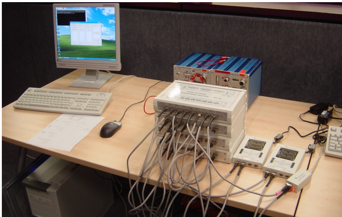
Figure 3 Four SpW-10X FPGA Prototypes Under Test
