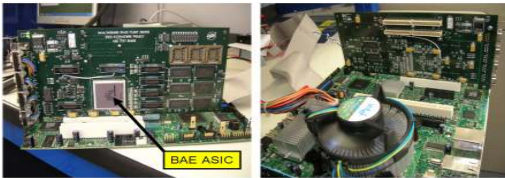
Figure 2. GOES-R SpaceWire Test Card in test station
