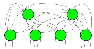
The cost of needing six eight-port switches to make a single full-bandwidth 16-port switch makes a strong argument for building switches with as many ports as possible. But, as we shall consider next, a single large switch is a large single point of failure.
