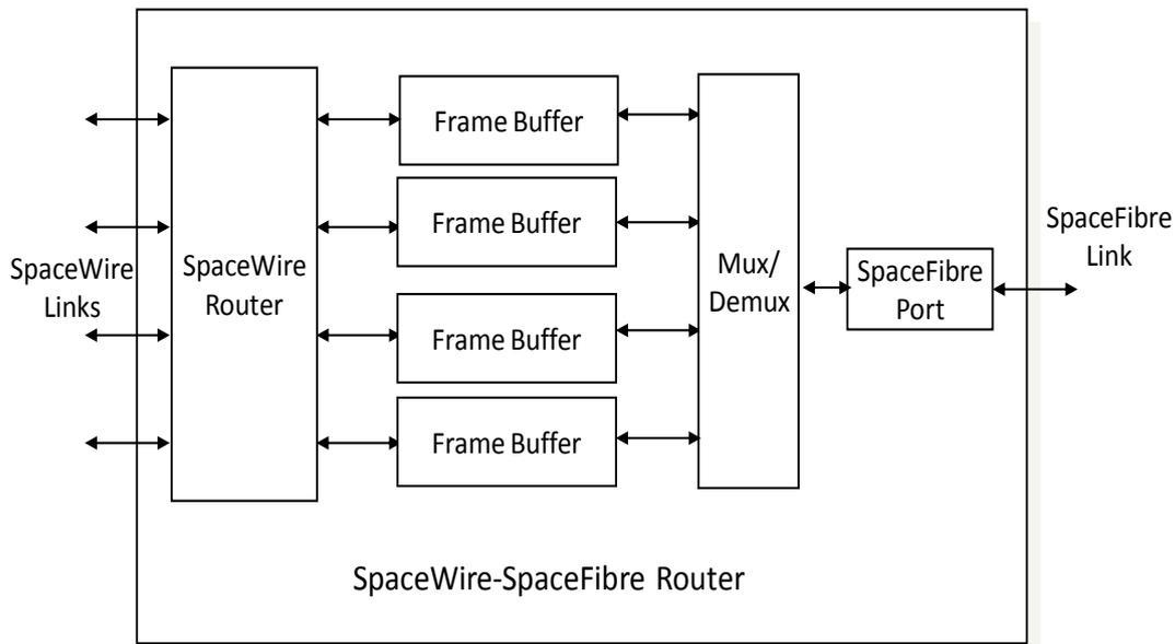
*Figure 3 SpaceWire-SpaceFibre Router*
